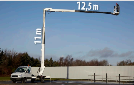
Perfectly vertical lower boom and horizontal upper boom**
