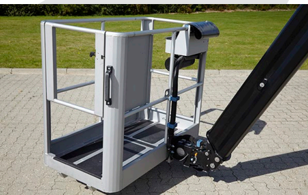
6 cm ground clearance below the end mounted cage
