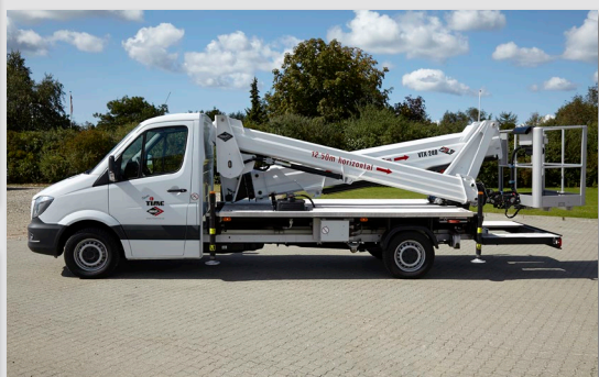
2 x 3 stage telescopic booms with patented 90° moveable knuckle in between
